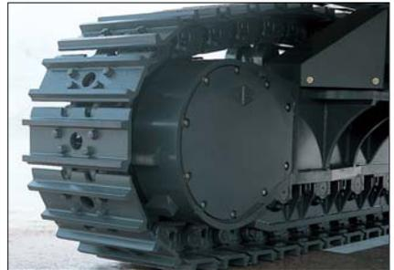
**Sturdy guards** shield the travel motors and piping against damage from rocks.
