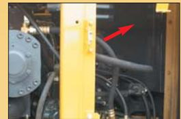
**Thermal and fan guards** are placed around high-temperature parts of the engine and fan drive.
